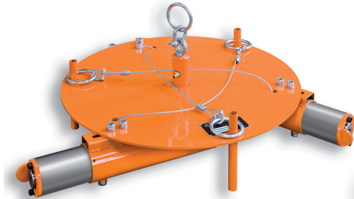
3-Arm-Automatik-Rüttler Ø 1000 - 1600 mm 3-arm automatic vibrator
